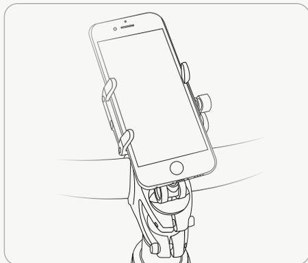
6. Fix the phone on the phone holder and tighten the knob.
