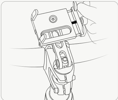
5. Unscrew the adjustment knob of the phone holder to the appropriate position.
