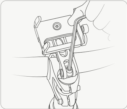
3. Fix it wrench (the inclination of the phone holder can be adjusted when the fixing screw is loose, and it will be fixed after tightengng).
