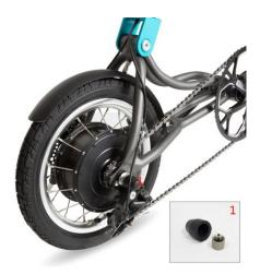
On the rear wheel axle, you will find a rubber plug and inside it a small metal switch that is inserted into the axle. This is essential to be able to activate the electrical system. Upon attaching it the electric motor will start working once you begin to pedal. For a better experience and to be able to control the help modes it is necessary that you download the APP Keyde.
