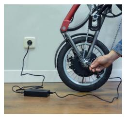
The Ossby Curve Electric can be recharged with the charger (provided with the purchase of the bicycle) by plugging it into any domestic electrical outlet. To connect it to the bike it is necessary to remove the rubber protector and the small metal switch located in the centre of the rear wheel axle simply by pulling them out. Once the connection is released, you just
